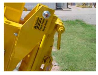
If the lever is in the position shown at right, the air will be shut off from the drill motor and will not run.
