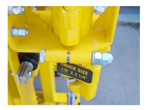
IMPORTANT: You must have the correct bit guide bushing to match the bit you will be using:
