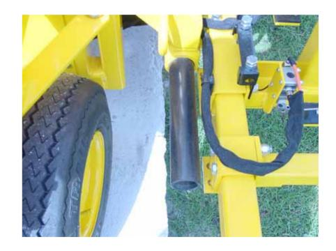
Unlock the red safety latch on the Raise & Lower Cylinders, and all of the individual carriage locks.
