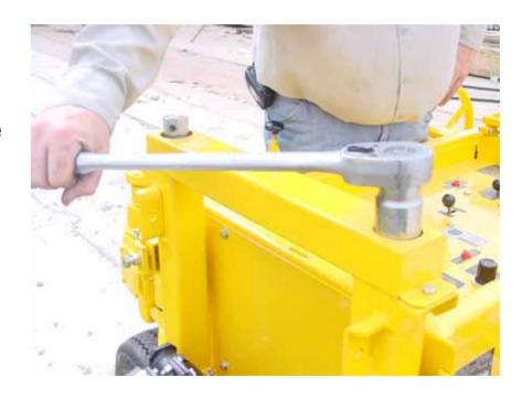
IMPORTANT: BEFORE LEVELING THE DRILL SYSTEMS, CONFIRM THE ANGLE REQUIRED. MANY TIMES THE DRILL SYSTEMS ARE NOT TO BE "LEVEL WITH THE WORLD", BUT SHOULD BE SET TO DRILL PARALLEL WITH THE TOP OF THE CONCRETE SLAB INTO WHICH YOU ARE DRILLING.
