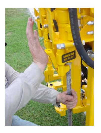
You may have to adjust the return stop rod so that the end of the bits clears the bit guide.
