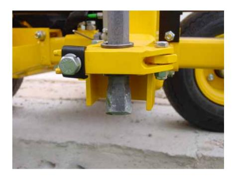
To adjust the stop rods, use the wrenches provided to loosen the stop rod nuts. Move the stop rod in the direction needed to the required location and re-tighten the nuts.
