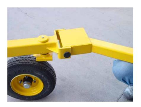
Pin the Hitch with the Hitch Pin Short into the hole of the Hitch Support.
