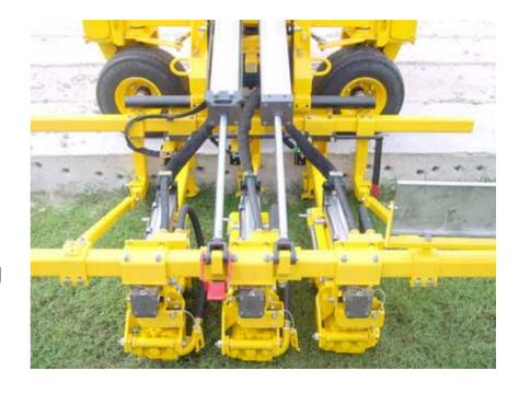
To slide a drill system one way or the other to reach the required drill spacing, you must first loosen the 5" frame clamps on each end of the feed bar. Loosen all four ½" lock nuts on each frame clamp until you can slide the feed bar.
