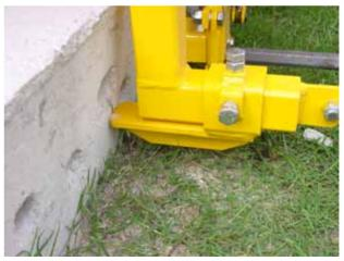
Place the feed lever into the "in" position. All of the drills will move forward until the bits contact the concrete slab.
