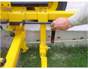
Attach the Hitch Support to the main frame by clamping it with the Frame Clamp onto the 3" square tube wheel frame support on the side at which you wish to tow the air compressor
