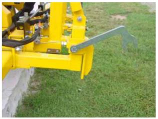
Place the proper bushing into the bit guide; one half in the upper bit guide and one half in the lower bit guide. Close bit guide, swing the swivel bolt back onto the bit guide, and tighten.
