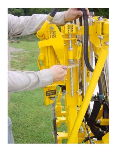
If you are using 2-piece H-thread bits, you may also have to adjust the guide plates (on the 210-3 SRA) or the guide wheels (on the 210-4 SRA and 210-5 SRA).
