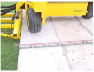
NOTE: THIS ADJUSTMENT WILL BE REQUIRED ANYTIME YOU HAVE BEEN DRILLING HORIZONTAL HOLES, AND NOW WANT TO DRILL STRAIGHT VERTICAL HOLES, OR VICE VERSA.
