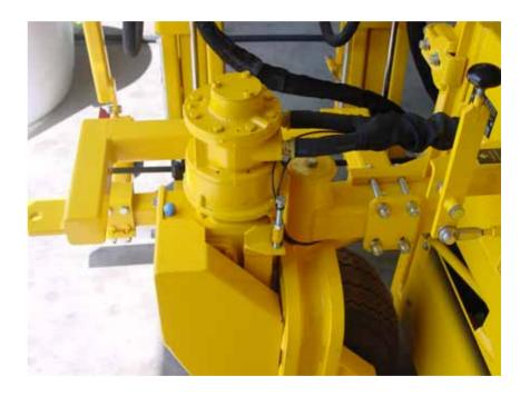
Depending on which kind of hitch is on your air compressor, bolt on the Compressor Mount and wheel assembly onto the air compressor hitch.
