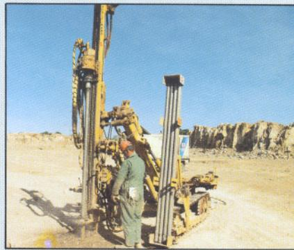
The CM-351 is a compact, powerful rig for drifter or downhole drilling of 64-140-mm (2 1/2 to 5 1/2") blastholes. Fixed-length boom. Its 2.2-m (7'3") width makes it easy to transport.
