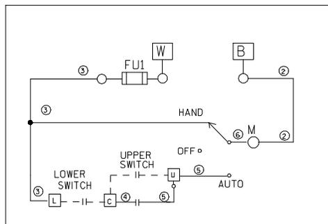
Figure B-6. Control Box 27511-105 Elementary Wiring Diagram
