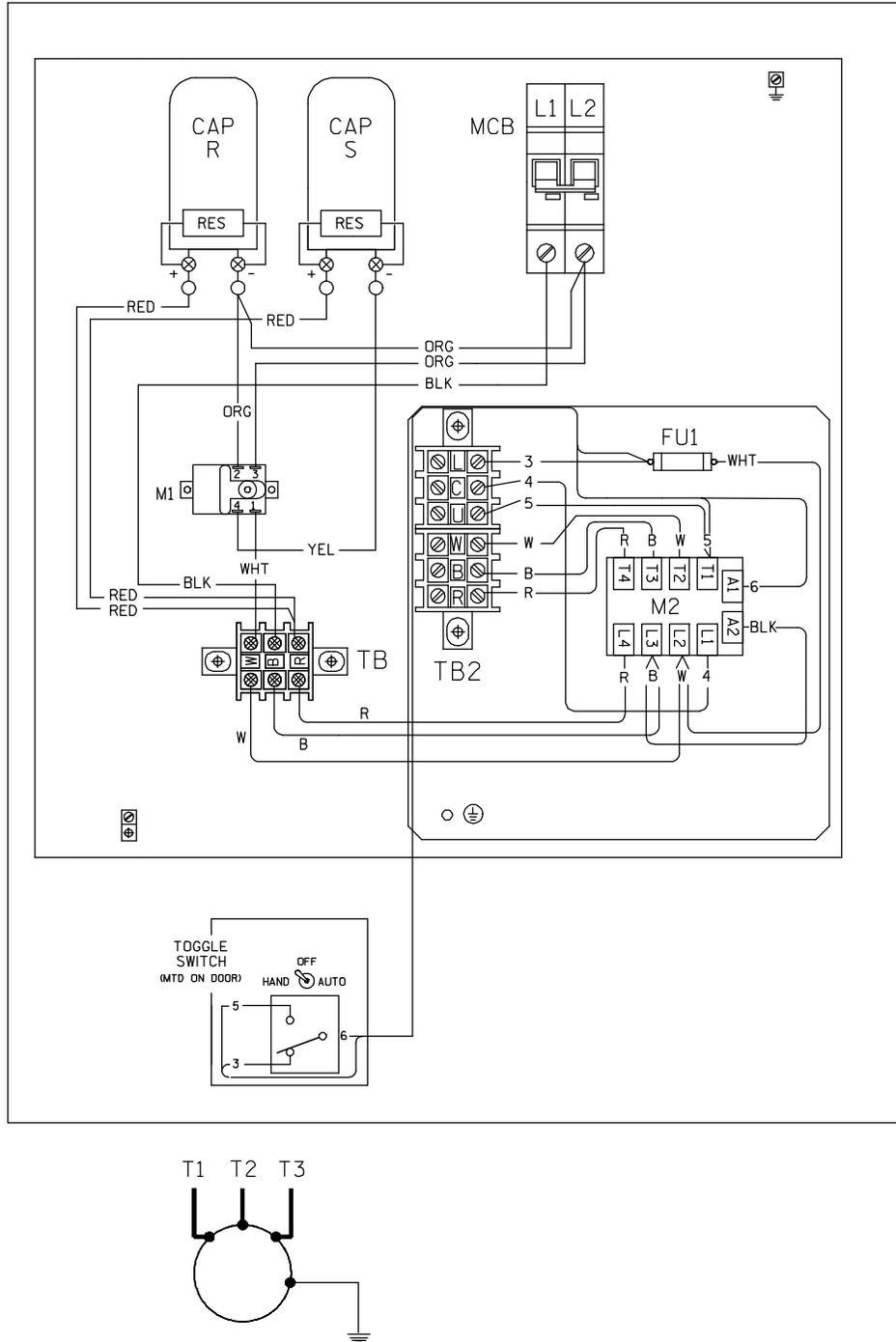
Figure B-5. Control Box 27511-105 Pictorial Wiring Diagram
