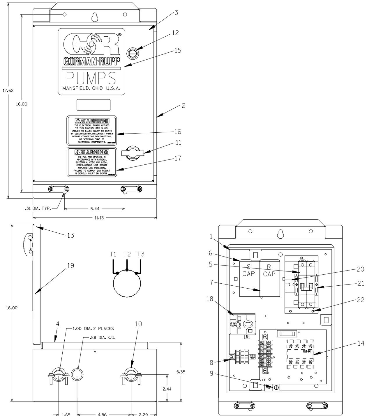
Figure 1. 27511-101, 27511-102, 27511-103, 27511-104, 27511-106 And 27511-107 NEMA Type 3R Control Box Dimension
