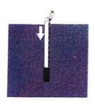
1. Insert splitting rods into holes.
