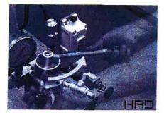
5. After that, for pistons going down, turn a control lever to the right(LOW).
