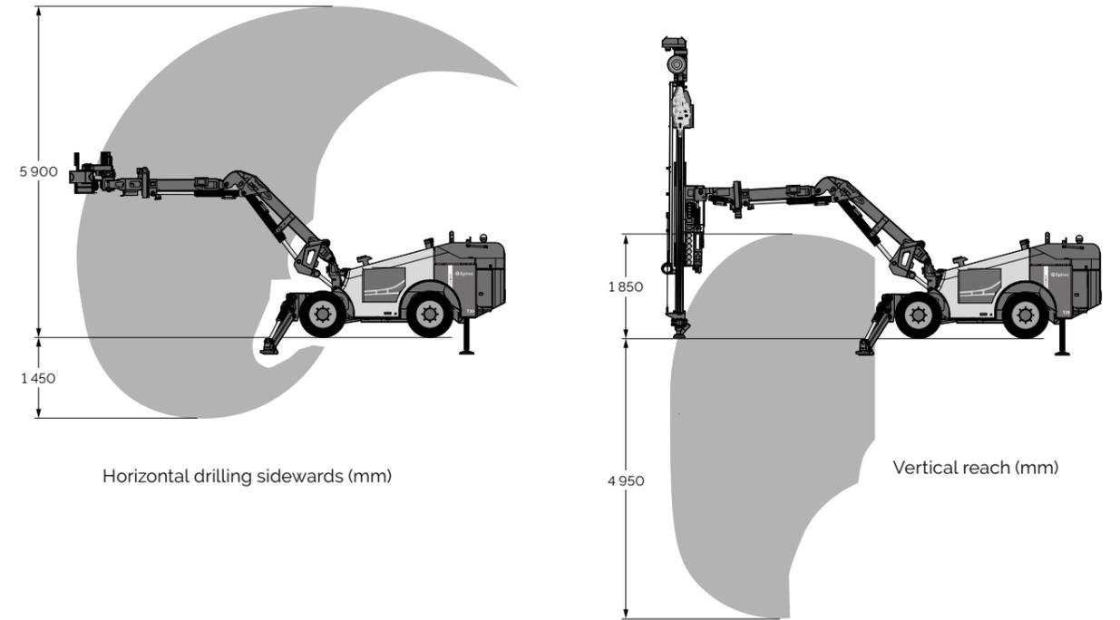
Horizontal drilling sideways (mm)
